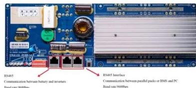
RS485 Communication between battery and inverters
